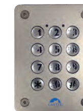
CLAVIER AUTONOME BRAILLE Standalone coded keyboard with backlit (blue) keys with Braille diameter 16 mm - 2 relays REF 330.0200 > Led and operating buzzer > Stainless steel vandal proof front panel > Flush mounted > Programming through the front panel via a master code > Dimensions 135 x 100 x 2.5 mm (Flush-mounted with flush box D 40 mm) > 140 x 105 x 60 mm (surface-mounted with optional surface box - REF 330.0150 -) > Power supply 12V not included
