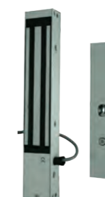
VENTOUSE ENCASTRE 300KG 24V Magnetic lock flush mounting standard compliant NFS61937 REF 320.1200 > Holding power 3000N > Length 230 mm > Width 38mm > Depth 27mm > 24V
