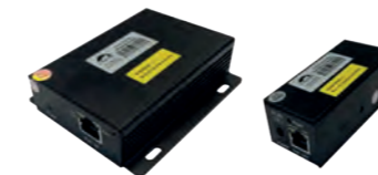
IP 2 WIRES CONVERTER Allows to connect a remote IP equipment on two wires. Made of 1 module "receiver" installed upstream and connected to the switch and 1 module "transmitter" installed downstream and connected to the remote IP equipment. REF 310.5000-1
