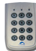
CLAVIER AUTONOME AV Zamak standalone coded keyboard (IP65 - IK10) with 2 relays - 1 buzzer REF 330.0050 > Blue backlight keys - 3 Leds > Tamper function > Programming through the front panel via a master code > Capacity: 100 user codes > Dimensions 120 x 36 x 83 mm > Power supply 12/24V 0.25V not included
